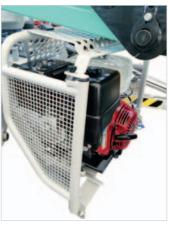
Strong protective engine structure for an increased impact protection.
