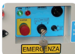
Ground control panel, intuitive and well protected from accidental bumps.
