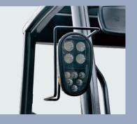
ne new efficiency lighting system nploys LED illuminant and new type flector to reduce energy consumption, prove significantly illumination reformance and prolong work time
